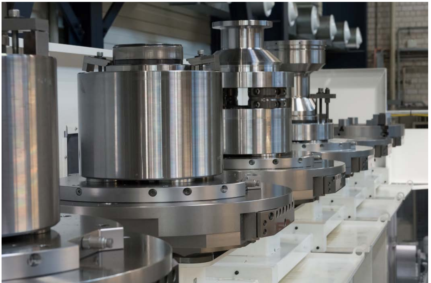
AMF zero-point clamping system in use on a milling-grinding centre with pallet. The zero-point system is the standard interface here on all machine pallets.
