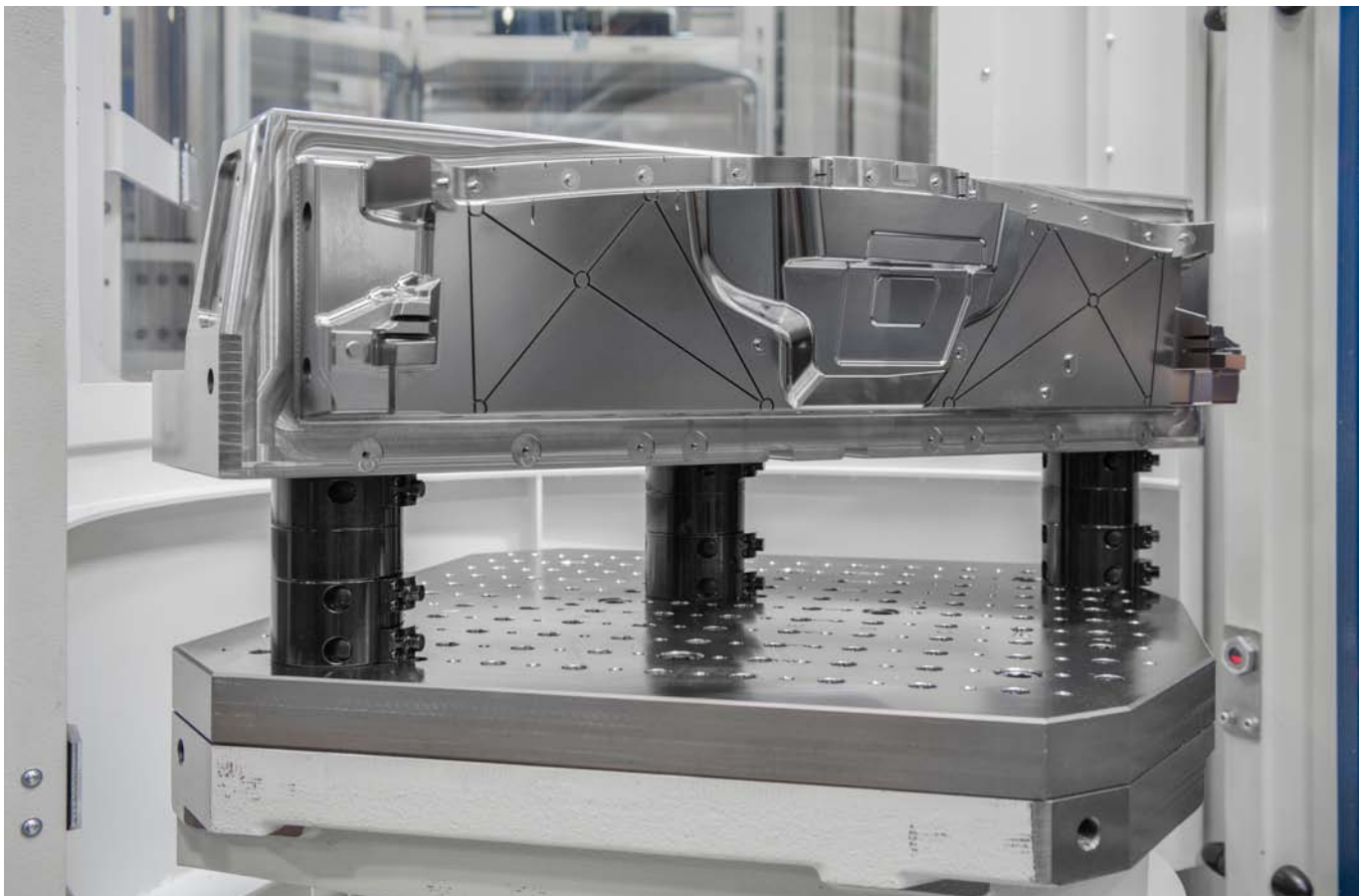
Modular mechanical zero-point clamping system in tool and mould making. The different clamping heights required can be easily adjusted using the standardized construction kit system.
