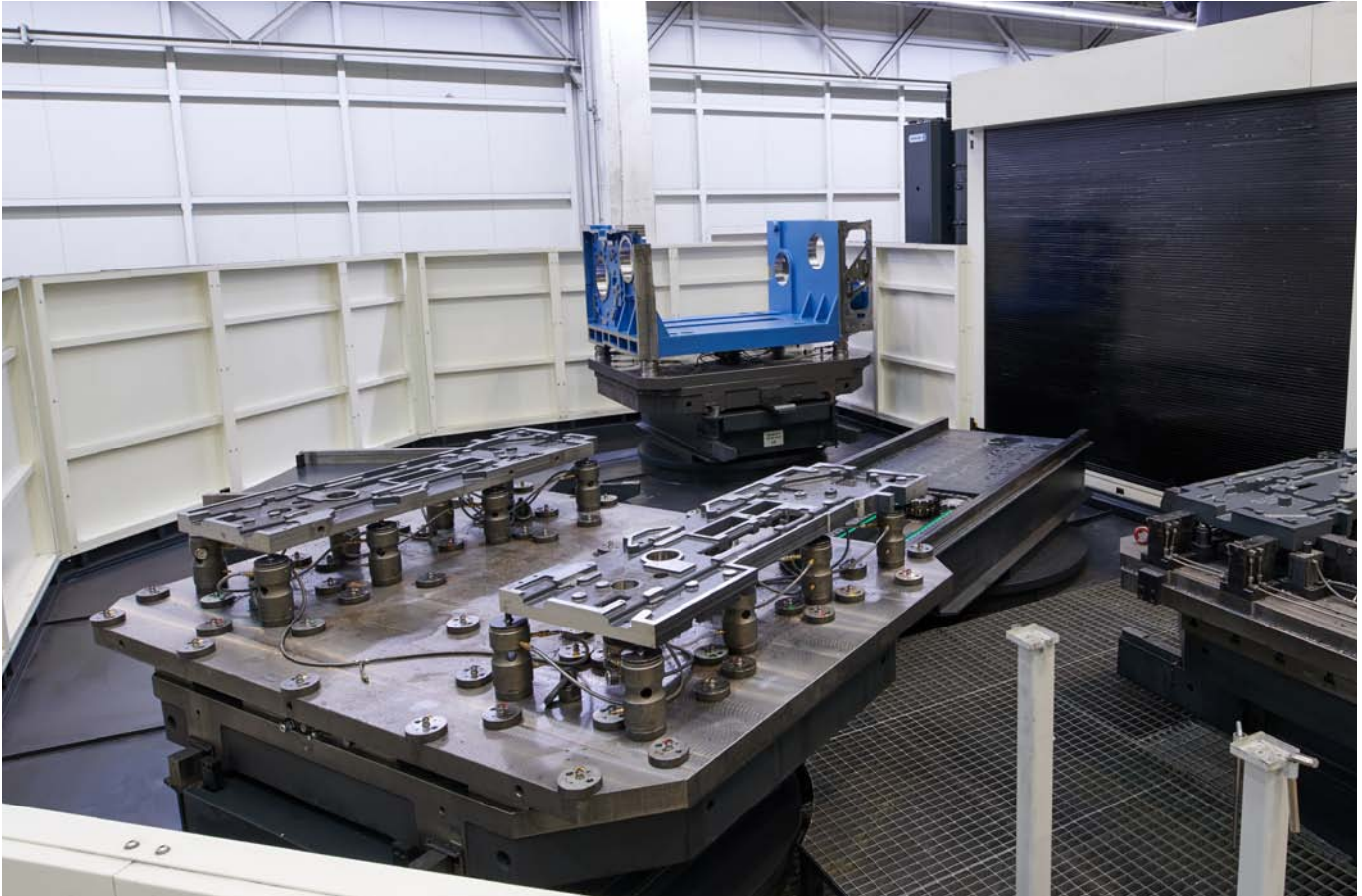
The zero point clamping towers are flexibly adapted to the respective workpiece by simply repositioning them. Colour coding ensures safe, repeatable clamping.
