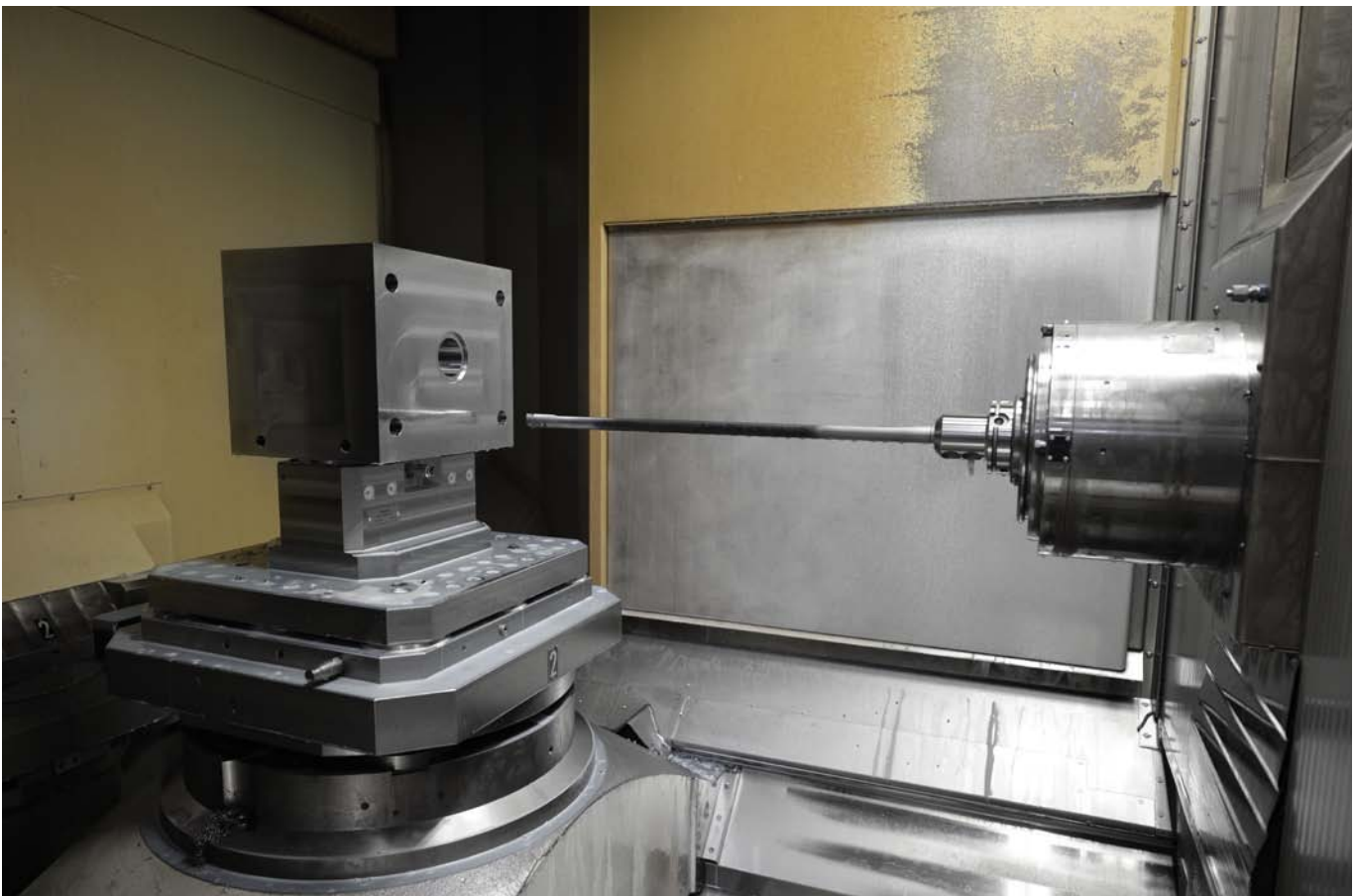
The large holding forces and repetition accuracy of the AMF - zero-point clamping modules are especially important for the precision of the deep-hole drill holes.
