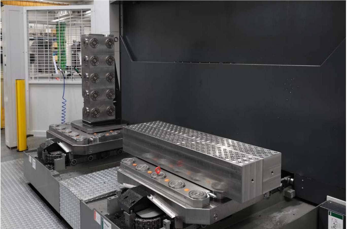
The large holding forces and repetition accuracy of the AMF - zero-point clamping modules are especially important for the precision of the deep-hole drill holes.
