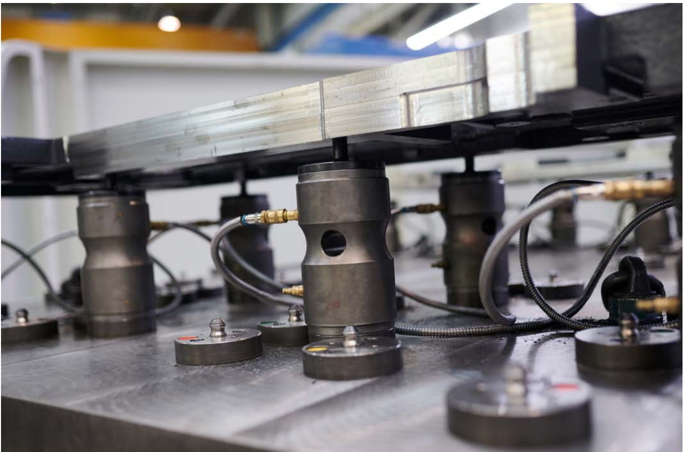
The zero point clamping towers are flexibly adapted to the respective workpiece by simply repositioning them. Colour coding ensures safe, repeatable clamping.
